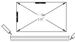
Center of frame should be 3/16" higher than jamb sides sag.
